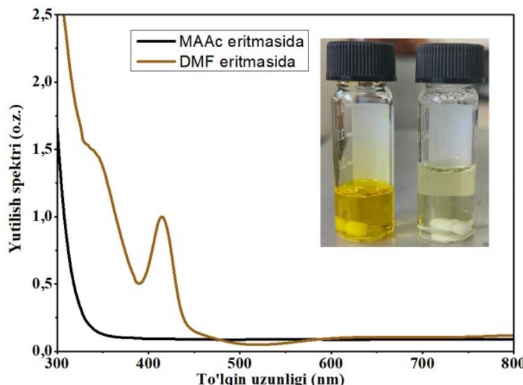
**Figure 1.** Absorption spectra of  $\text{CsPbI}_3$  perovskite active layers prepared in DMF and MAAC solvents before heating.
