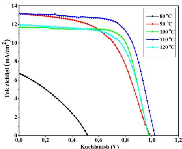
**Figure 8.** Current-voltage characteristic graph of  $\text{CsPbI}_3$  PSCs prepared in MAAC solvent at different heating temperatures.
