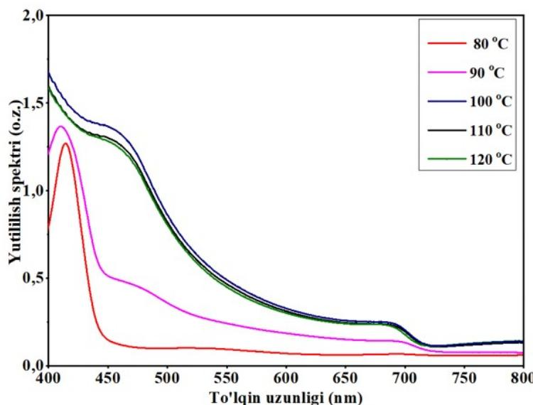
**Figure 2.** Absorption spectra of perovskite active layers prepared from a perovskite solution in DMF solvent after thermal heating at different temperatures.
