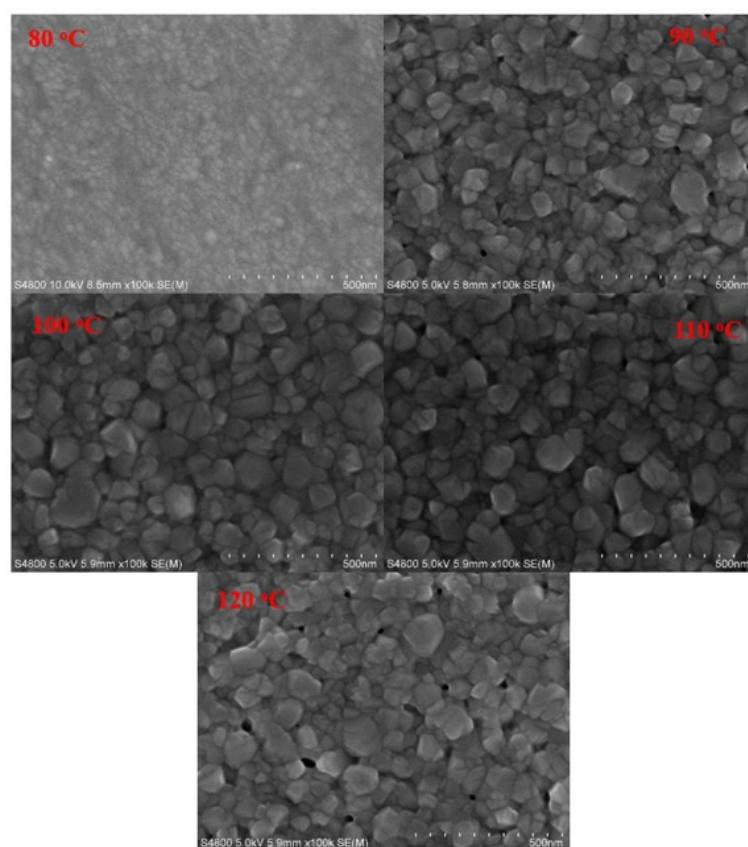
**Figure 5.** SEM images of perovskite active layers prepared in DMF solvent and heated at different temperatures.
