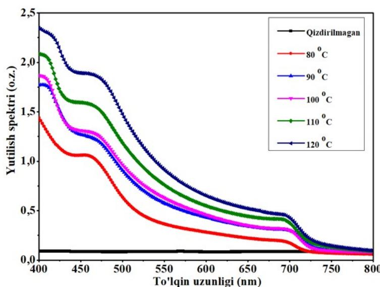
**Figure 3.** Absorption spectra of  $\text{CsPbI}_3$  perovskite active layers prepared using MAAC solvent and thermally heated at different temperatures.
