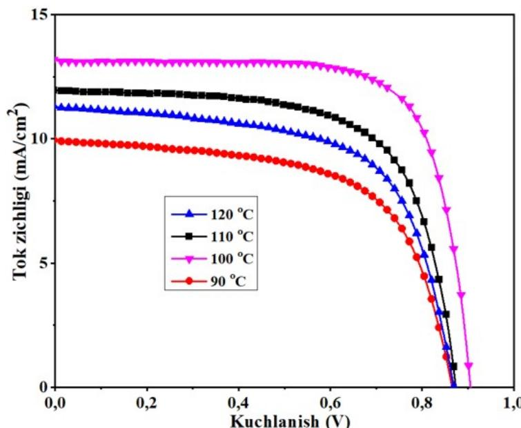
**Figure 7.** Current-voltage characteristic graph of  $\text{CsPbI}_3$  PSCs prepared in DMF solvent at different heating temperatures.
